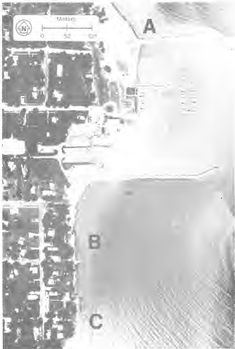
Figure 3. Lexington Harbor, 16 June 1980. A is the accretion area at shoreward end of north breakwall; B and C indicate erosion along the shoreline south of harbor.
